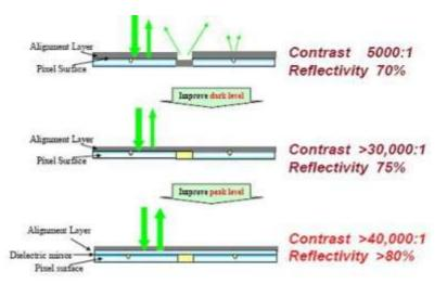
Figure 10. Process refinement of D-ILA leading to higher efficiency and contrast ratio
