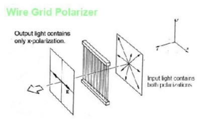
Figure 13. Schematic of Wire Grid Polarizer operation
