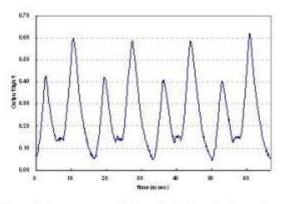
Figure 8. Projection output light at the 128 gray level as a function of frame time. There are two light pulses per frame.
