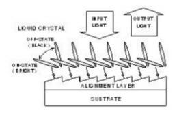
Figure 9. VAN LC alignment used in D-ILA devices
