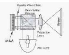
Figure 11. Optical Schematic of Basic D-ILA Projecto
