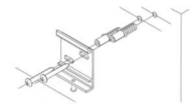
Insert the provided plastic anchor into the holes.
