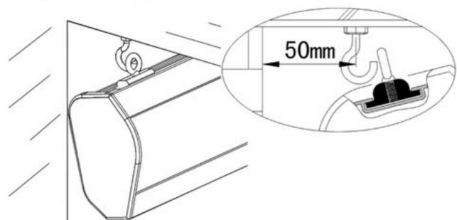
There is a 10mm clearance between the wall and the screen housing after installation
