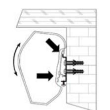
Hang the screen onto the wall mount bracket as shown on diagram
