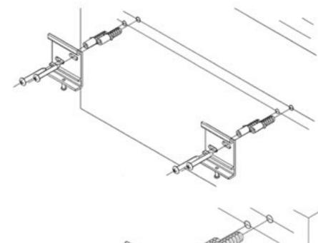
Mark 2 horizontal parallel lines on wall at desired height. Drill holes on wall According to the openings on wall mount bracket
