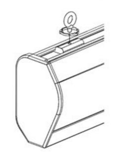
The "J" hook should in installed at least 50mm from the wall
