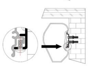
Afterwards tighten the securing screw, Prevention the screw comes out from wall mount bracket.
