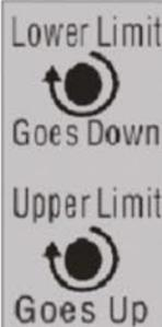
**Lower limit**—Adjust the stopping level of slat when fully extend. Turn "lower limit" switch in clockwise direction let the slat go closer to the ground.
