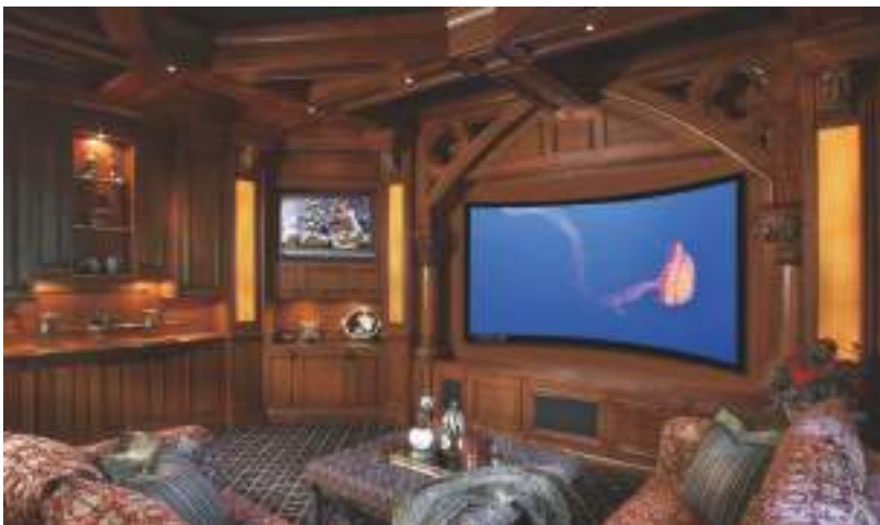
Use acoustically transparent perforated weave fabric front projection materia, It allows speaker placement behind while allowing an exceptional acoustically transparent performance.
