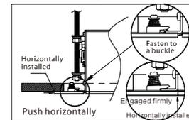
**Note:** If it's not horizontally installed screen end cap, can use a clip to easily disassemble end cap for reinstallation.
