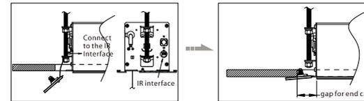
① Connect with IR sensor to the IR interface.
