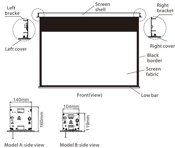
A-Type ceiling cut out dimension: cut out length Lt = Screen Total length - 26mm; cut out width 150mm, height  $\geq 160$ mm;
