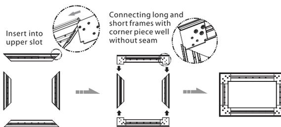
**Note:** after assembly of frames, please pat slightly position A and B, please check below. If there is seam appearing, please loosen screws on corner piece for adjustment until it is seamless before tight the screws again.
