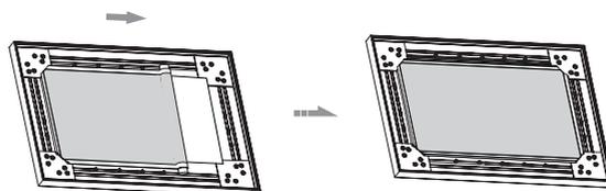
Lay the screen material flat and insert the tension rod from the edge of screen material. Please see below:
