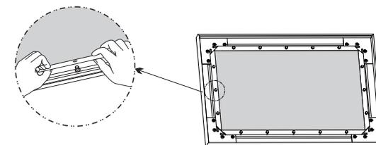
**Note:** If screen material is unflat or has wrinkles, please make slight adjustment on position of snap lugs.
