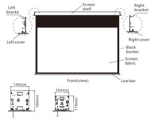
Type A: Side(view) Type B: Side(view)
